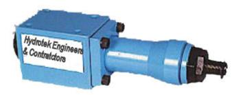
Four Pressure ranges- 25,50,100,200, bar with primary pressure rating to 315 bar Two options for- With set screw and Lock nut Pressure setting by screw adjustment.
